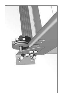
Insert dowels and fasten the end bracket to the wall using tapping screws and washers.
