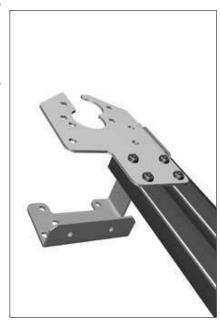
Place on both horizontal tracks the connected construction of the end support bracket for drum behind and safety device fastening bracket for drum behind fastening. Fasten the assembled bracket to the double horizontal tracks using bolts 8X16 with semi-round head and tighten them with nuts.
