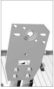
Fasten the end support bracket to the double horizontal tracks using bolts and nuts.
