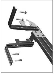
Fasten the multi-purpose bracket to the ceiling using 2 tapping screws.
