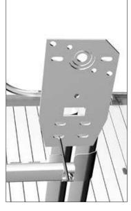
Place the end support bracket against the horizontal tracks on the outside. Mark the holes in the tracks for bracket fastening using perforation in it.
