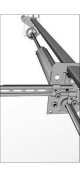
Fasten the assembly to the ceiling using brackets (the bracket type depend on the lintel height).
