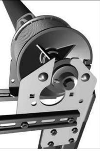
Fasten the end plate with bearing to the end support bracket for drum from behind using 2 bolts with semi-rounded head (M8X16), fix the bolts on the close to the lintel or far from the lintel slots (relatively the embrasure) depending on the installed drums.
