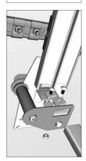
Position and fix the cable guiding roller for drum behind together with the mounting angle for horizontal lath on the end support bracket using a bolt and a nut. Position and fasten the C-profile using mounting angles, lock plates and bolts with semi-rounded head M8x25 and suitable nuts.
