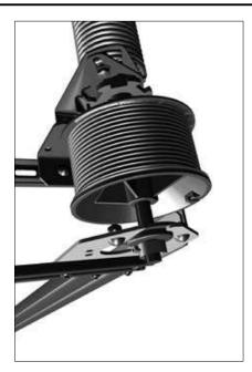
Fasten the spring failure safety device to the end support U-shaped bracket using 2 set of fasts (bolt 10X25, nut M10, spring washer 10).
